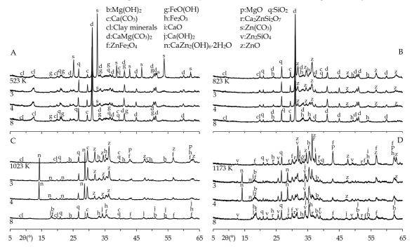
Fig. 5. XRD patterns of heated ore samples and the residues obtained after leaching of the heated samples at indicated NaOH concentrations (mol/dm³) (Only intense peaks are labeled for clarity.)
