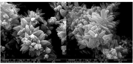
Fig. 7. SEM images of the solids precipitated from pregnant solutions obtained by leaching of the ore sample (left) and the ore sample heated at 723 K (right) in 4 mol/dm<sup>3</sup> NaOH solution
