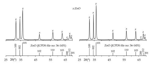
Fig. 6. XRD patterns the solids precipitated from pregnant solutions obtained by leaching of the ore sample (left) and the ore sample heated at 723 K (right) in 4 mol/dm<sup>3</sup> NaOH solution
